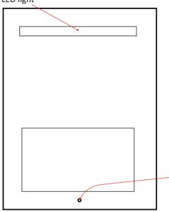
Push the control button to switch on/off the led light.
